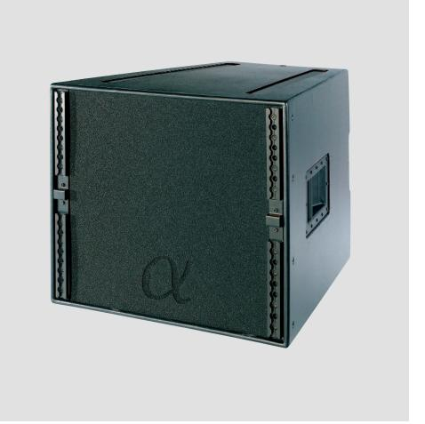
The ALPHA M8 is an advanced high power, medium-Q Mid/HI module that has the same form factor as the high-Q M3, allowing user selectable dispersion characteristics appropriate to the application. The M8 uses two exponential horn loaded 10" MF drivers and a constant directivity horn loaded 3" HF driver giving 75° x 45° dispersion, the horn may be rotated with the wider dispersion in the horizontal or vertical plane.
