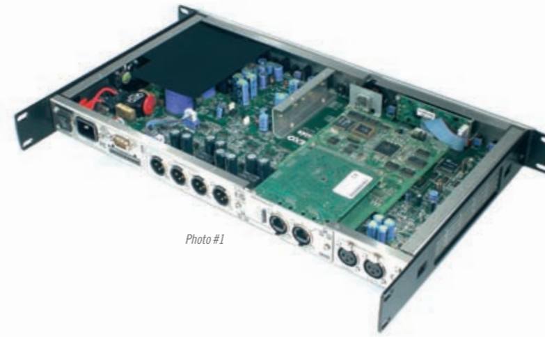
Photo #1: NX242, with top removed, fitted with NXtension-ES4 Expander Board. (Notice twin Cat5 connections on NXtension-ES4 back panel)
