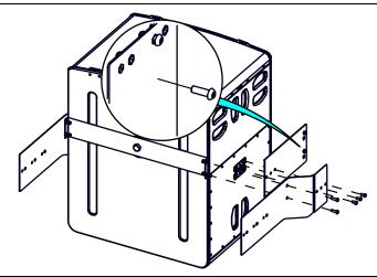
Tighten the screws. Secure with the 4 provided M10x30 screws.
