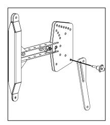
INSERTING PIN - FLOWN SETUPS
