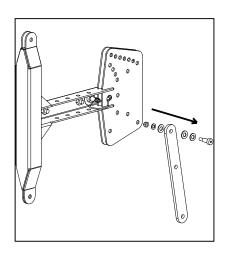
REMOVING STANDARD LINK BAR
