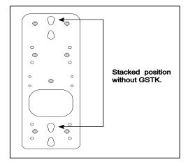
Connect bottom LS18 or GEO S12 to GPT-GSTK Ground stacking device with 4 8x20 quick release pins;
