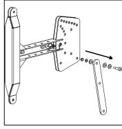
REMOVING STANDARD LINK BAR
