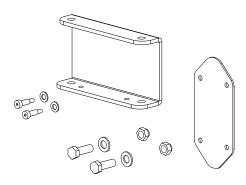
MARNING: Screws must be secured using Loctite 243™
