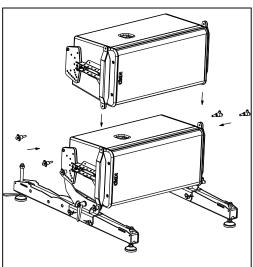
Once the assembly is completed, rotate rear or front GEO S12 ground stack device adjustable legs to definitive tilt angle, ensuring that +/-10° is never exceeded on bottom GEO S12.
