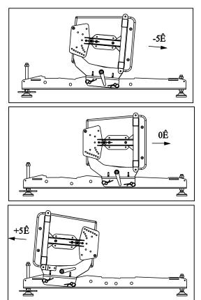
Connect the reinforcement bar to the supporting beams according to required tilt angle configuration using 2 axis per side; secure the axis with provided "R" clips;
