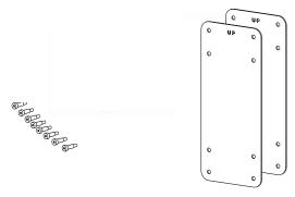
MARNING: Screws must be secured using Loctite 243™
