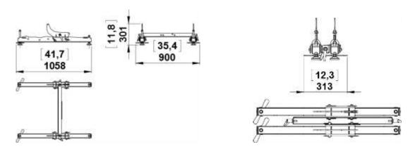
Depending on tilt angle – negative, null or positive - to be achieved, there are three positions to connect above assembly to the supporting beams.
