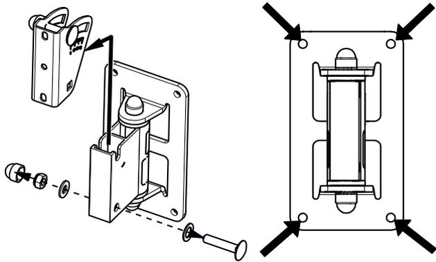
Screw speaker plate to Nexo Speaker (use only screws provided with Nexo Speaker – 10mm wrench).
