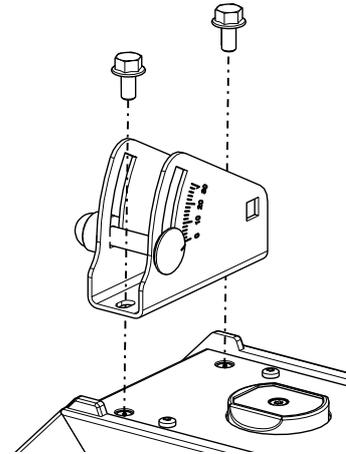
Place the speaker holder with Nexo speaker into the wall bracket. Fix by tightening bolted assembly.
