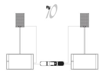
NXAMP4X2<sub>MK2</sub> powering 1 X PS10R2 and 1 X LS600 Sub per side
