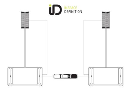
NXAMP4X1<sub>MK2</sub> powering 1 X ID24 and 1 X IDS110 Sub per side
