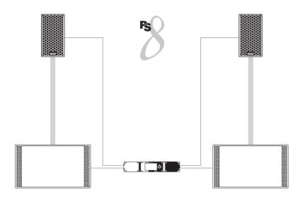
NXAMP4X1<sub>MK2</sub> powering 1 X PS8 and 1 X LS400 Sub per side
