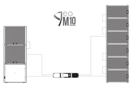
NXAMP4X2<sub>MK2</sub> powering 3 X MSUB15 (one in cardio mode) and 6 X GEO M10
