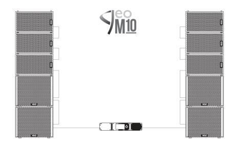
NXAMP4X2<sub>MK2</sub> powering 3 X GEO M10 and 2 X MSUB15 per side
