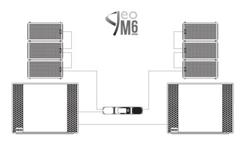
NXAMP4X1<sub>MK2</sub> powering 3 X GEOM6 per side and 2 X LS18 in mono bridge
