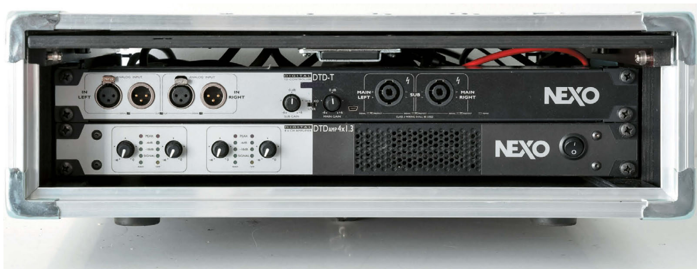
Amp rack with Nexo's DTD 4x1.3 amp and DTD controller
