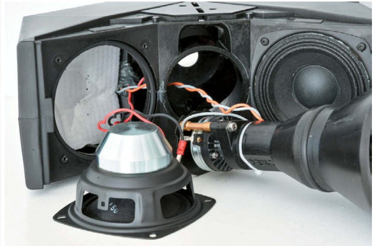
The ID24's 4" bass/mid-range unit with neodymium magnet; after releasing the adjustment knob, the tweeter can be completely pulled out towards the front. The small neodymium driver operates with a 1" coil over the horn's 1/2" opening
