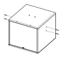
Place the assembly below the frame plate. Pay attention to the mounting direction, see the mark on the top frame.
