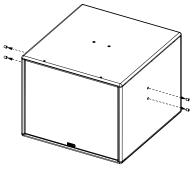
Place the assembly below the frame plate. Pay attention to the mounting direction, see the mark on the top frame.
