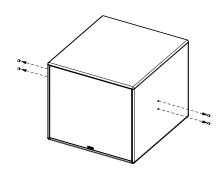
Assemble the Plates on each side of eLS18 using the M10x25 screws.
