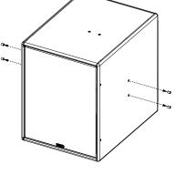
Assemble the Plates on each side of eLS600 using the M10x20 screws.
