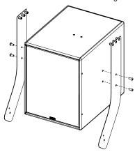
Remove the screws on both sides of ePS8.
