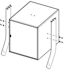
Place ePS10, fasten with M10x25 and M6x25
