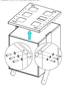
Remove the screws on both sides of ePS10.
