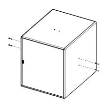
Assemble the Plates on each side of eLS18 using the M10x25 screws.
