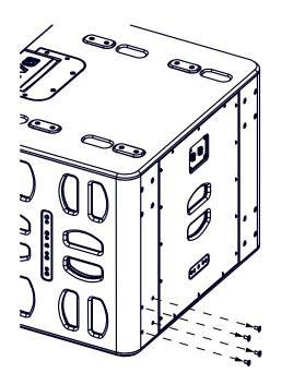
Fit the caster and secure it with the 4 notched screws supplied.
